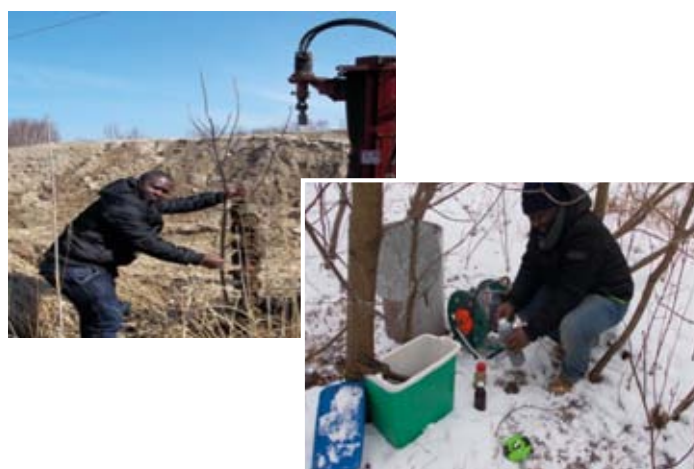
Figure 10: Site characterisation and collection of groundwater samples for screening evaluation of PRmB system for mixed contaminants
