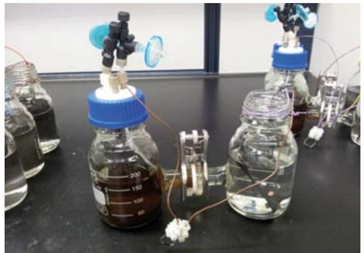
Figure 4. New microbial fuel cell reactor design
