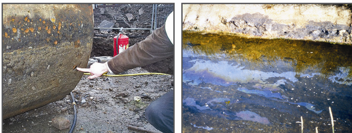
Figure 1.1. Example of LNAPL releases showing a leaky underground storage tank (left) and LNAPL impact to a surface-water receptor (right) (Courtesy of N. Clarke and M.O. Rivett respectively).
