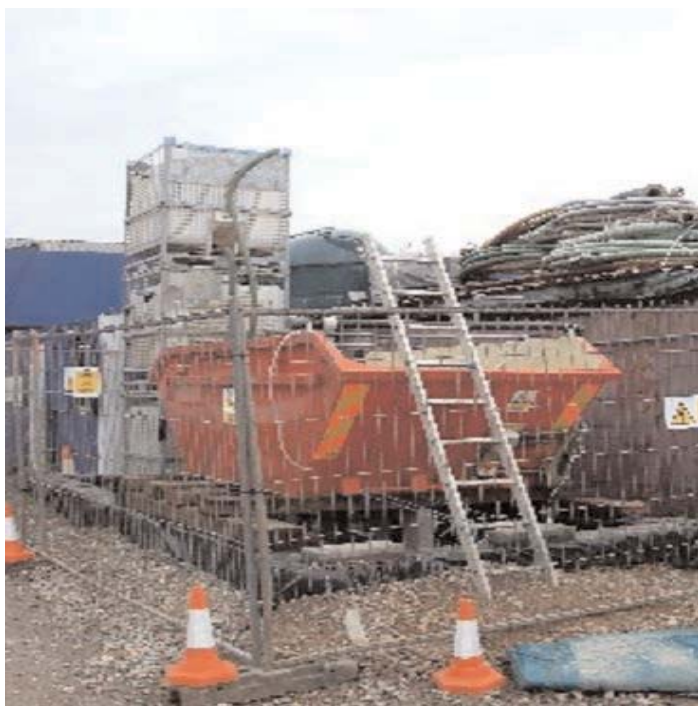
Fig. 2: The Treatment Container (TC) fabricated for the experiment. The connected white tower structure behind the TC holds electro-osmotically mobilized aqueous solutions from which 5 L samples were taken for purification prior to de-alkalisation.
