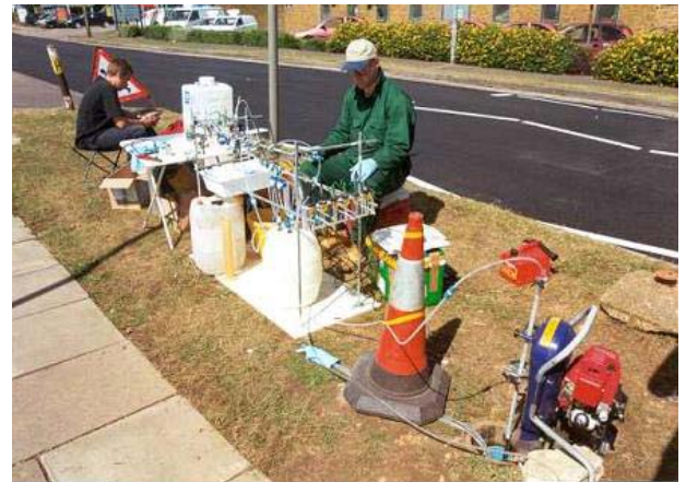
Apparatus used to collect groundwater samples from multilevel samplers
