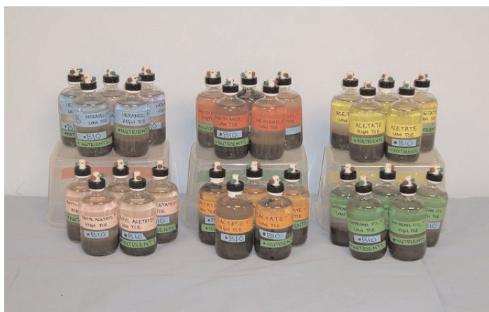
Figure 1. Subset of the more than 130 microcosm experiments conducted with site soil and groundwater (CL:AIRE Research Bulletin 6).
