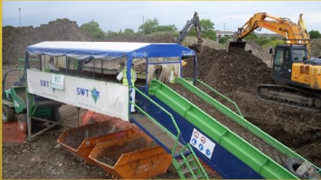
Typical picking station used to reduce the concentration of asbestos fragments in recycled soils.
