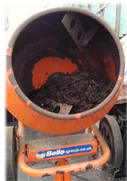
Mechanical preparation of soil to ensure heterogeneity (© ReCon Soil)
