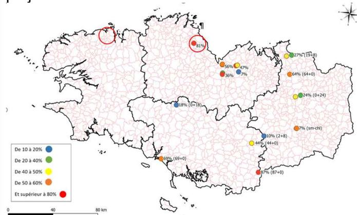
Figure 1. Samples with XRD analysis in Brittany containing swelling minerals (smectite etc.) - XRD analysis carried out as part of the mapping of the shrinkage and swelling hazard in Brittany.
